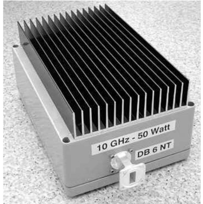
This x-band transverter was built for the 60 ft. dish at the AMSAT DL Bochum site to be used for EME and Tropo. The purpose is to get ready for the Mars mission and other deep space endeavors. The amplifier puts out 50 Watts on 10 GHz. The receiver has a noise figure of .65dB and the 144 Mhz input power required is 3 W
