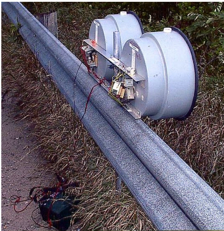
47 GHz set up. DB6NT, aimed at the Glen Arbor Cannery EN64xu from Miller Hill EN74at Lloyd NE8I
