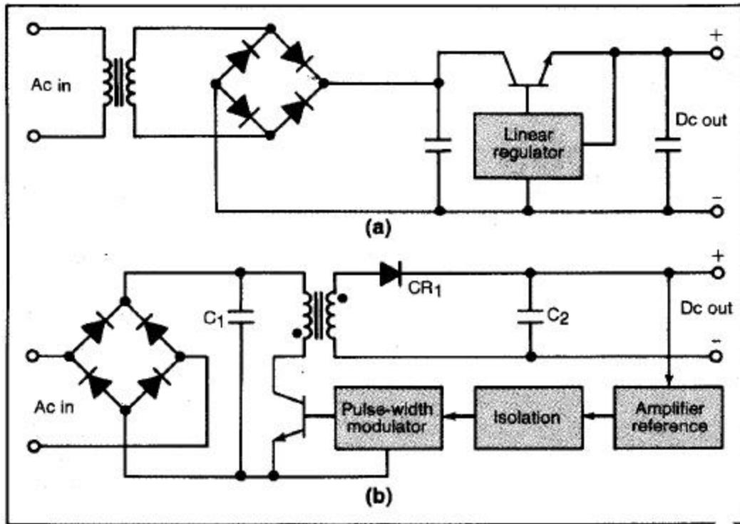
1. The analog, or linear, method (a) uses a dissipative transistor to regulate the dc output voltage or current. The digital, or switch-mode, method (b) regulates by adjusting the pulse width of a square wave derived from chopping the dc rectified from the ac power mains. The regulated pulses must then be rectified again and filtered before voltage can be delivered to the output.
