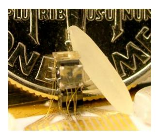
While this clock is amazingly tiny, its performance is limited and it is subject to frequency drift with temperature as well as from contamination in the tiny gas cell; it drifted about  $2x10^{-8}$  (that's about 2 Hertz at 100 MHz) per day. NIST has done another prototype using a Rubidium cell rather than Cesium, and it performs better (the red line is the Rb clock; black is the original Cs version):
