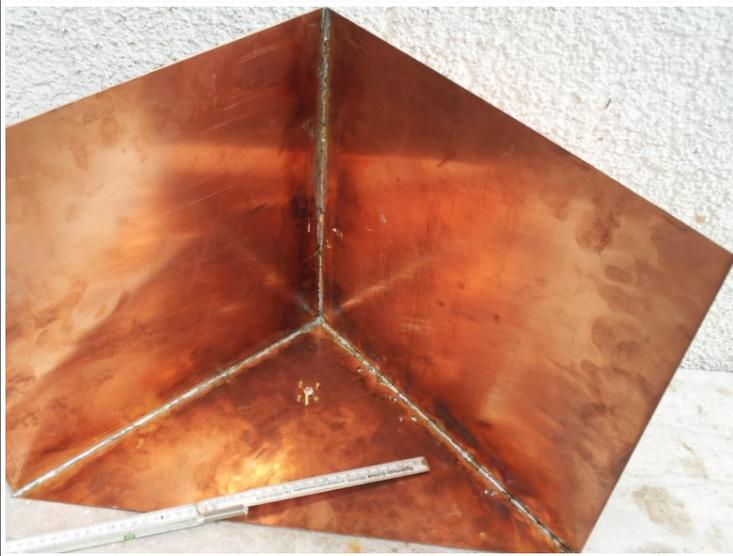
This 3-sided corner reflector provides about 18 dBi gain!!! The driven element is a simple  $\frac{1}{4}$  vertical, and requires one additional grounded director element for a good match. The three sides are about 2.8 square. The ground-plane side can be reduced to a triangle, but that lowers the gain to about 16.5 dBi. Mounting requires a special bracket, as the main lobe extends at a 45° angle from all three surfaces. For 1296 MHz the sides are about 26" long.
