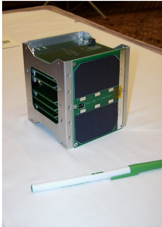
A PC-board for a cubesat, cubesat w. circuit boards, 2 solar panels .... photos by Keith, KB1SF
