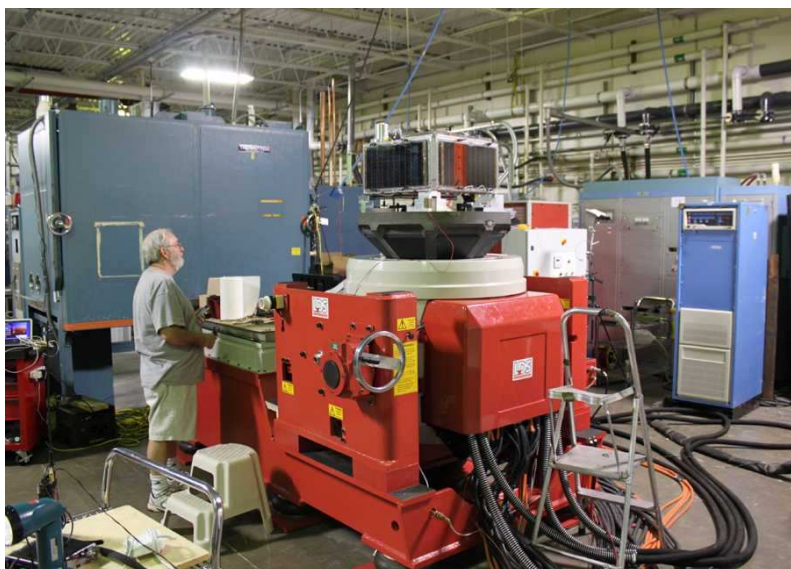
AMSAT BOD member Lou McFadin, W5DID, prepares the ARISSat-1 flight model satellite for vibration testing at a contractor facility in Orlando, Florida.
