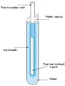
However, the absolutely most exact temperature reference is the "triple point" of water – that is, where water exists in all three phases (solid, liquid, and gas) simultaneously. This equilibrium occurs at a temperature of exactly 273.16° Kelvin, or 0.01° Celsius, and a partial pressure of 6.1173 millibars.
