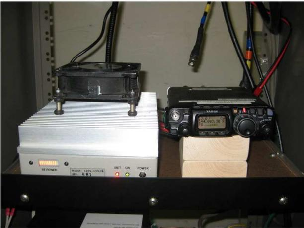
Temporary Beacon setup includes an FT-817 keyed by a PIC keyer to generate a two-meter signal. That signal is feed into a Down East Microwave 1296 20W transverter. There is 900 feet of 7/8" feedline going to the antenna so we don't get much power at the antenna. Maybe 1 to 2 watts at best.
