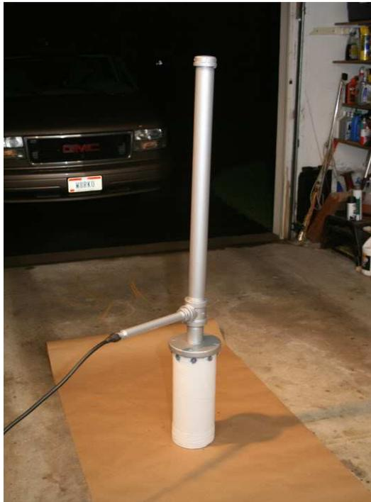
1296 Beacon Antenna after painting. Note the antenna will hang upside down in the white fiberglass cylinder on the bottom.
