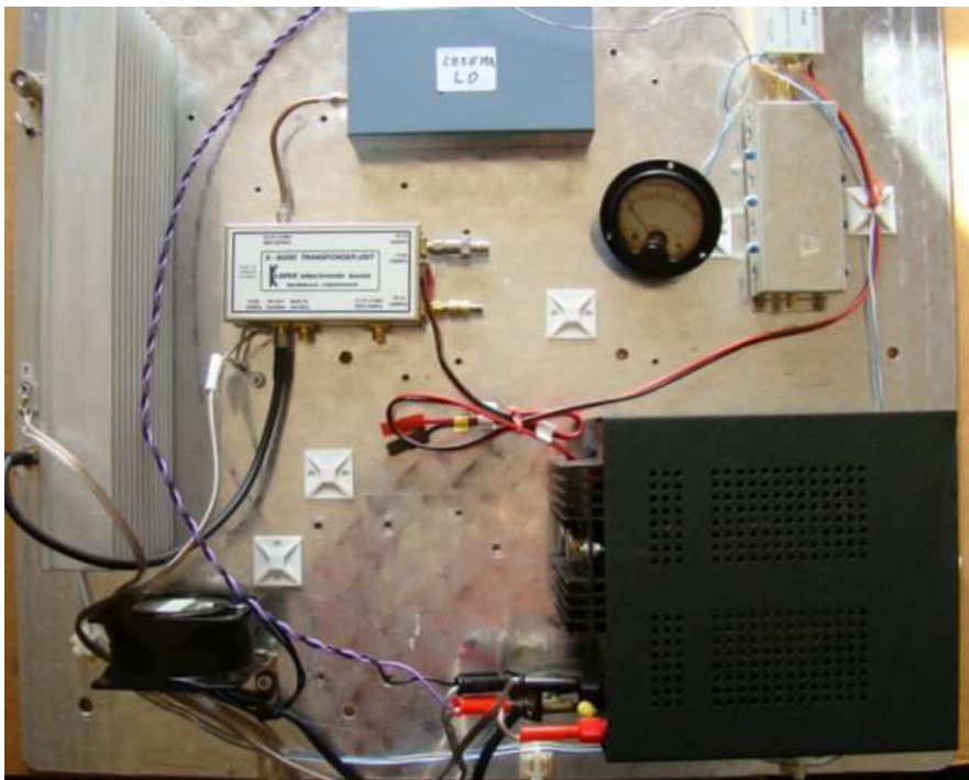
Transponder, left the 30W 13cm PA, right, power supply, above output meter and 23cm preamp and filter, left center, transponder core 70cm and 23cm converters to 13 cm, above that, new local oscillator /2838MHz
