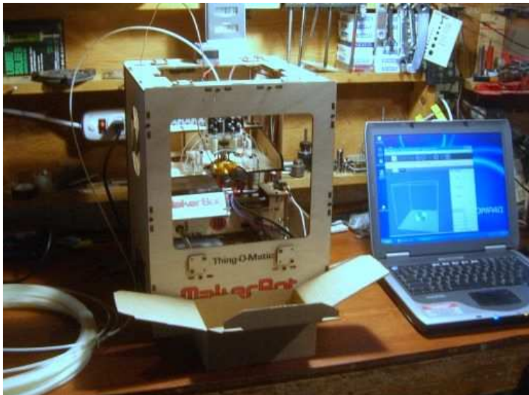
1 lb roll of 3mm(1/8") plastic, sturdy wood frame with printing mechanism inside, laptop to control printing
